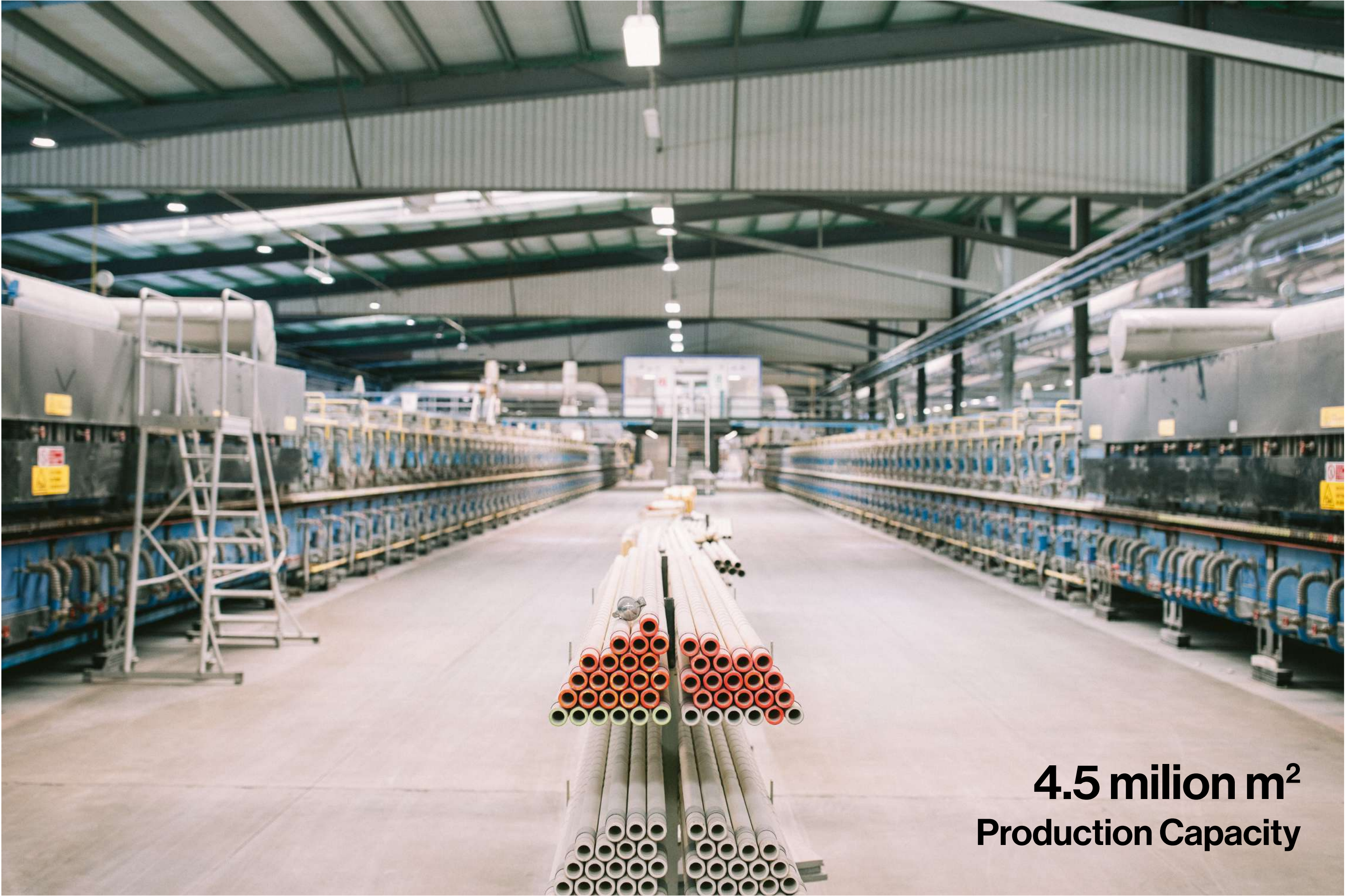
Ceramic rollers on which our porcelain slabs run through the kilns at our production site in Vetschau (Germany).
